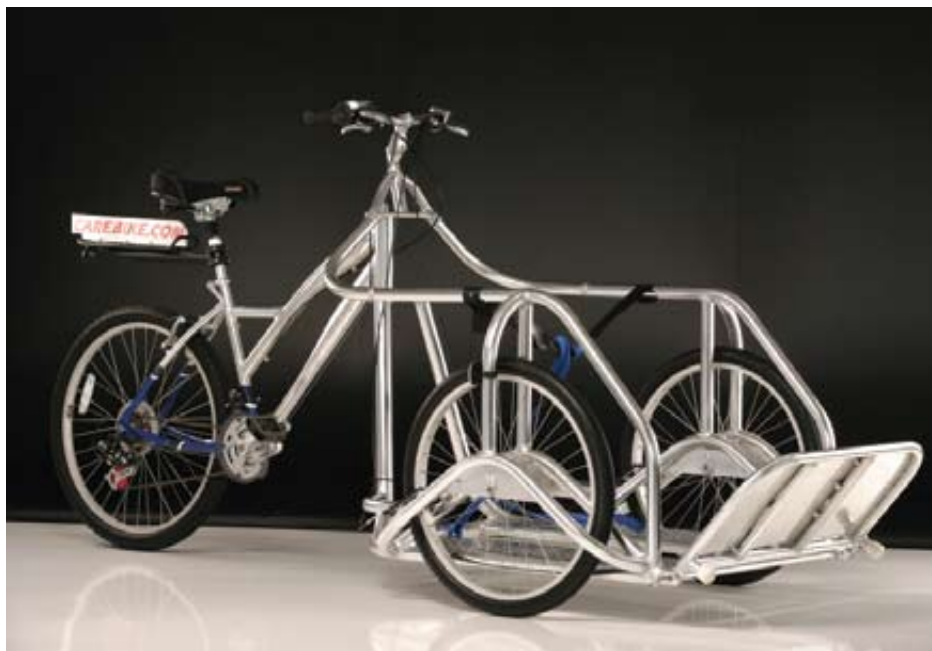
CAREBIKE is a reverse tricycle, designed to hold a wheelchair up front.
